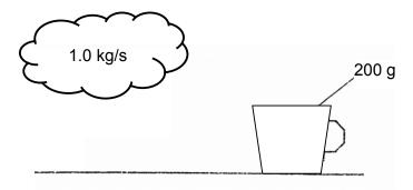
If the specific heat capacity of coffee is 4.0 kJ/kg°C and that of air is 200 J/kg°C, compute the time necessary to cool the cup of coffee to 50 °C.
