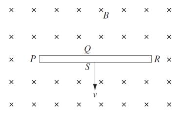
Which side of the conductor has the greatest concentration of electrons?
