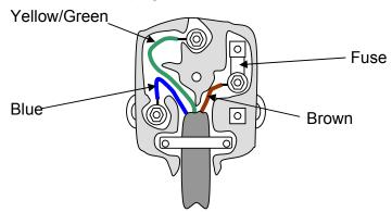
If the brown wire carries a current of 4 A when the appliance is switched on, what would be the currents in the yellow/green and blue wires?
