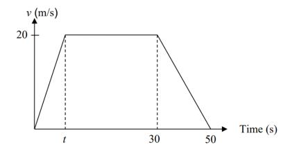
The diagram shows the speed-time graph of a car.
