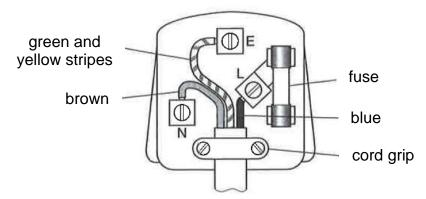
(a) State in what way the mains plug has been wired wrongly.
