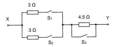
**19** When switches S<sub>1</sub> & S<sub>2</sub> are closed, what is the effective resistance of the composite circuit?
