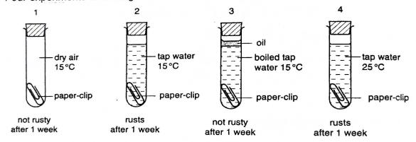
Which experiment(s) can be used to show that water is needed for iron to rust?
