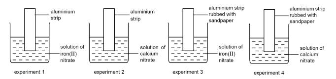
In a laboratory, some experiments involving aluminium were set up.
