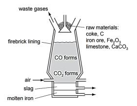
(a) The coke reacts with the oxygen in the air to form carbon dioxide.
