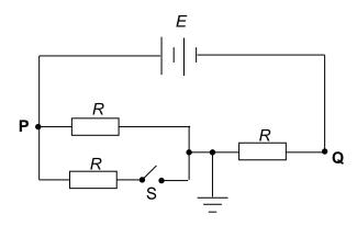
What happens to the electric potential at **P** and at **Q** when the switch S is closed?
