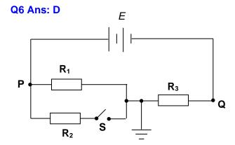
When switch S is closed,  $R_1$  and  $R_2$  become a parallel arrangement. Thus, p.d. across  $R_1$  and  $R_2$  decreases while p.d. across  $R_3$  increase since e.m.f. remains the same. As the potential at the earthed junction is zero, the potential at P becomes less positive, hence decrease while the potential at Q becomes more negative (hence, decrease).
