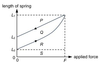
Which combination of areas give the work done by the force to extend the spring from  $L_0$  to  $L_1$  and which area gives the increase in potential energy of the particles in the spring when its unstretched length is increased from  $L_0$  to  $L_2$ ?
