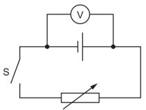
When switch S is open, the variable resistor is adjusted to have a value of 8.0  $\Omega$ , the voltmeter reads 1.5 V.
