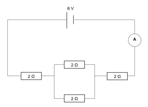
(a) Determine the effective resistance of the circuit.
