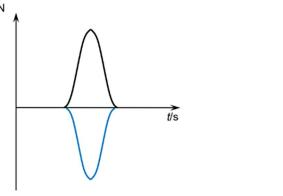
By Newton's third law, the force by the hammer on the pile is equal and opposite in direction to the force by the pile on the hammer.
