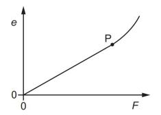
The point P is the elastic limit. Plastic deformation occurs when the rod is extended beyond point P, causing it to be permanently distorted.
