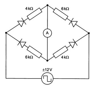
The ammeter records the mean current in the central link between the upper and lower parts of the network. The diodes have either zero or infinite resistance.
