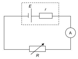
R is set at two different values and the corresponding currents I are measured using an ammeter of negligible resistance.
