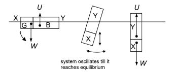
Weight *W* and upthrust *U* creates a net moment on the system which causes the system of blocks to rotate anticlockwise and oscillate.
