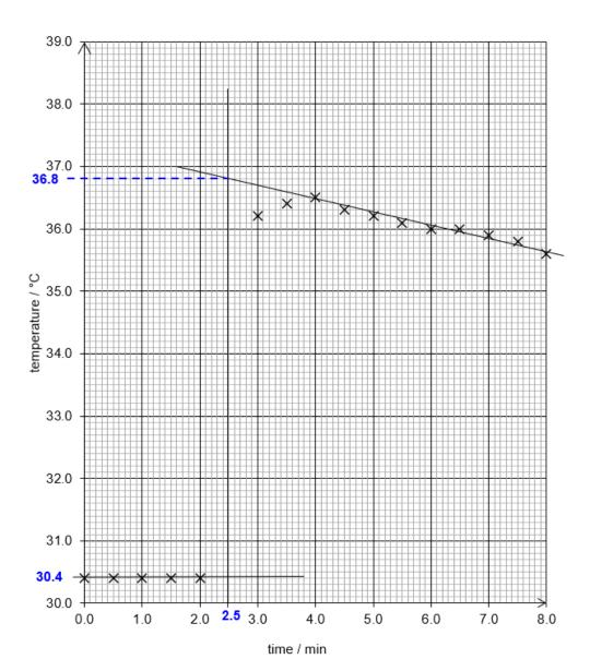
1(b)(iii)  $T_{\text{min}} = 30.4 \,^{\circ}\text{C}$   $T_{\text{max}} = 36.8 \,^{\circ}\text{C}$  $\Delta T = +6.4 \,^{\circ}\text{C}$
