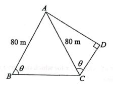
(a) Show that the total length, L metres, of material required to build the above bridge component is given by  $L = 160 + 240\cos\theta + 80\sin\theta$ . [2]
