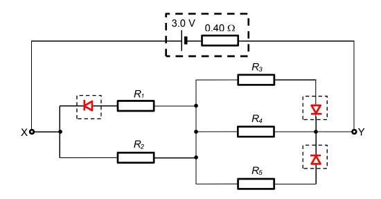
[M1] Correct orientation (Not accepting just arrows, students should at least draw the <u>triangle</u> to indicate direction of allowed current flow)
