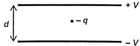
The separation of plates is  $d$ . The droplet is observed to be stationary when the upper plate is at potential  $+V$  and the lower potential  $-V$ .
