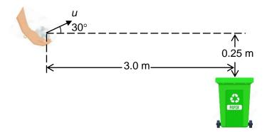
The horizontal distance between the centre of mass of the ball and the centre of the trash bin is 3.0 m, while the vertical distance between them is 0.25 m. The ball is shot at an angle of  $30^{\circ}$  above the horizontal, with an initial speed *u*.
