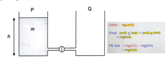
When the tap is opened, water flows from P to Q until the water level in both containers is the same. How much potential energy is lost by the water?
