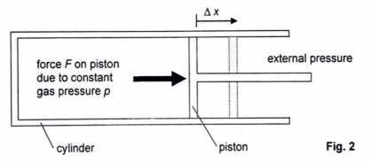
As the gas expands, a force F is applied on the piston by the gas molecules to move the piston against the external pressure (also constant). The work done by force F in displacing the piston of cross-sectional area A through a small distance  $\Delta x$  is the work done by the gas<sup>2</sup>,  $W_{gas}$ .
