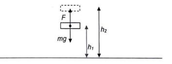
Work done by F in displacing the center of mass of object vertically upward,
