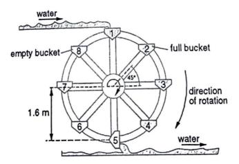
The distance between the centre of each bucket and the centre of the wheel is 1.6 m. When a bucket is at its highest point, the bucket is filled with a mass of 40 kg of water. The wheel rotates and the bucket is emptied at its lowest point. The wheel makes six revolutions per min.
