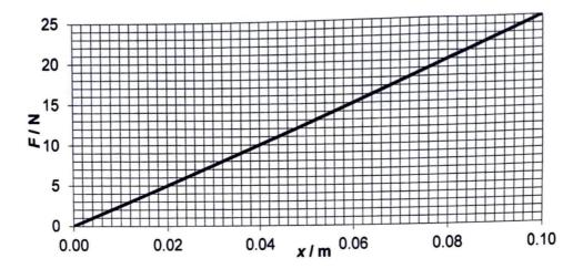
A load of 10 N is placed on the spring. How much additional elastic potential energy will be stored in the spring if it is then extended a further 0.040 m?
