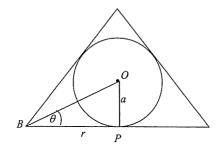
A right circular cone of base radius r is designed to contain a sphere of fixed radius a.
