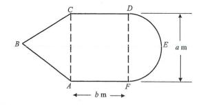
Suppose DF = a m, AF = b m, and the area of the field is fixed at 400 m<sup>2</sup>. Find, using differentiation, the values of a and b which give a field of minimum perimeter, giving your answers correct to 2 decimal places. [8]
