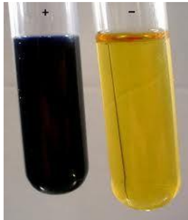
Fig. 2.7: Starch (tube on the left) gives a blue-black colour with iodine solution (brown solution).
