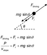
$$\theta = \sin^{-1} \left[ \left( \frac{P}{v_{\text{slope}}} - F_r \right) \left( \frac{1}{mg} \right) \right]$$
