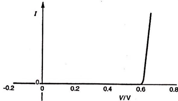
Describe, with the help of equations, how the resistance of this diode depends on the potential difference  $V$  across it.
