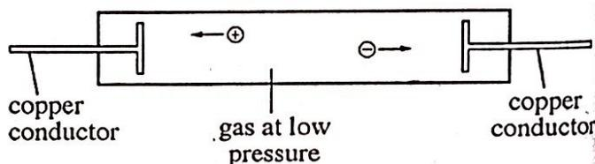
In this case, the copper conductors to the gas carry a current of 0.28 mA. The number of negative particles passing any point in the gas per unit time is  $1.56 \times 10^{15} \text{ s}^{-1}$  and the charge on each negative particle is  $-1.60 \times 10^{-19} \text{ C}$ .
