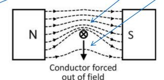
(b) Combined Fields Causing Force on Conductor
