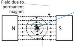
Field due to current-carrying conductor
