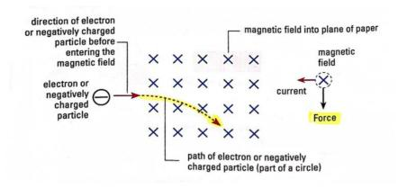
Paths are always similar to an arc of a circle as the force acting on the particles is always perpendicular to the direction of motion.
