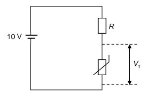
When the temperature of the thermistor is 20 °C, its resistance is 5.3  $\Omega$  and the potential difference  $V_{\tau}$  across it is 4.5 V.
