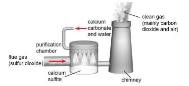
SO<sub>2</sub> reacts with calcium carbonate to form calcium sulfite (CaCO<sub>3</sub>) and CO<sub>2</sub>.
