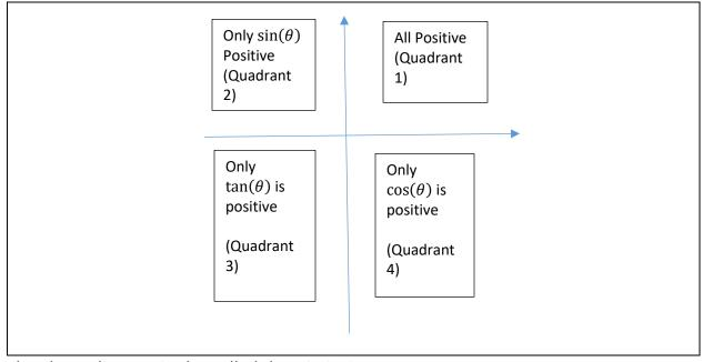
The above diagram is also called the ASTC Diagram.
