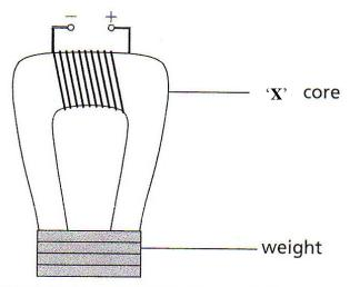
A student is experimenting with the use of several materials to be used as the core of the electromagnet. The table shows the data for four cores made from different materials. The relative permeability of a material is the measure of the degree to which the material can be magnetised or the ease with which magnetism can be induced in the presence of an external magnetic field.
