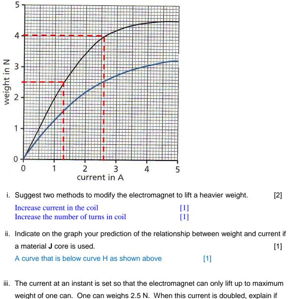
the electromagnet is able to lift two cans at the same time?[2]From graph, to lift 2.5 N can, current needed is 1.3 A. When current is doubled to 2.6A, weight of can to be lifted is 4.0 N.[1]The electromagnet is not able to lift 2 cans which weigh 5.0 N.[1]
