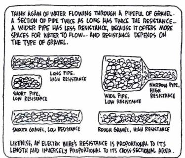
Every material has a characteristic resistivity. Good electrical conductors have low resistivities and insulators have high resistivities.
