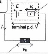
In the external load resistance R, power dissipated as heat,  $P_R = I^2 R = I V_R$
