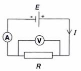
The ammeter measures the current flowing through the component and the voltmeter measures the p.d. across it. The resistance can thus be determined using  $R = \frac{V}{I}$
