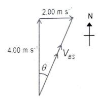
Velocity of the boat relative to the shore is 4.47 m s<sup>-1</sup> in a direction 26.6 ° East of North.
