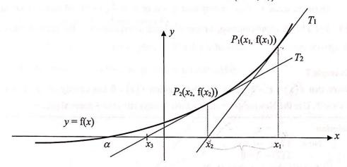
The gradient of the tangent  $T_1$  at  $P_1(x_1, f(x_1))$  is given by  $f'(x_1)$ . The tangent  $T_1$  intersects the x-axis at  $(x_2, 0)$ .
