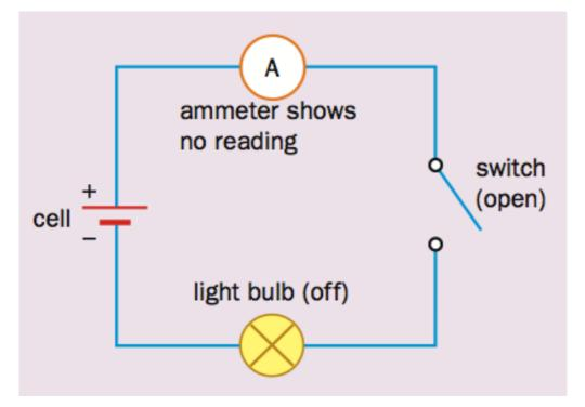
An open circuit is a circuit in which current is unable to flow due to breaks in the circuit
