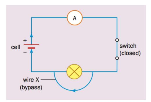
A closed circuit allows electricity to flow through without any interruptions (but in this diagram, the bulb will not light up due to the least resistance being on the bypass)
