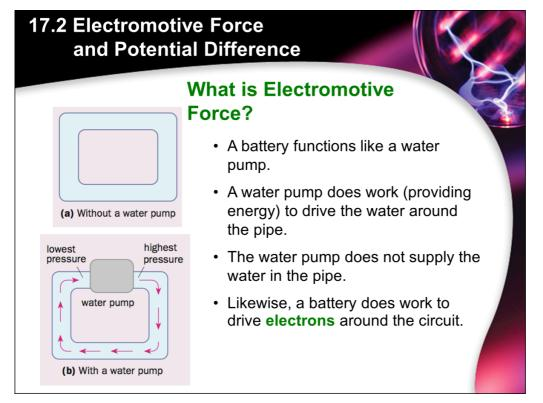
The electromotive force (e.m.f) of an electrical energy source is defined as the work done by the source in driving a unit charge around a complete circuit.
