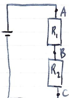
$$V_{AB} = \frac{R_1}{R_1 + R_2} V_{AC} \quad V_i = \frac{R_1}{R_1 + R_2} V_s$$
