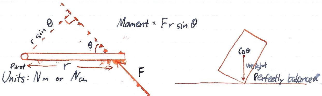
If the ~~vertical~~ vertical line through an object's CoG falls within its base, it can return to its original position
