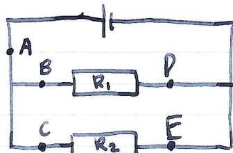
$$\begin{aligned} I_A &= I_B + I_C \\ \text{emf} &= V_{BD} = V_{CE} \\ \frac{1}{R_{\text{e}}} &= \frac{1}{R_1} + \frac{1}{R_2} \end{aligned}$$
