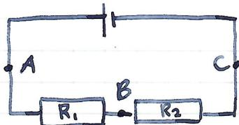
$$\begin{aligned} I_A &= I_B = I_C \\ R_{\text{e}} &= R_1 + R_2 \\ \text{emf} &= V_{AB} + V_{BC} \end{aligned}$$
