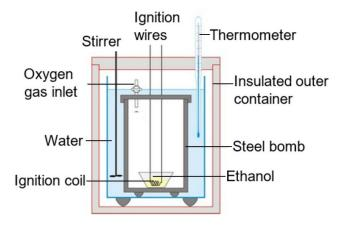
In the bomb calorimeter, the bomb was filled with oxygen gas at high pressure and was immersed into a container filled with water. The liquid ethanol was then ignited using ignition wires. The maximum temperature of the water inside the calorimeter was measured.
