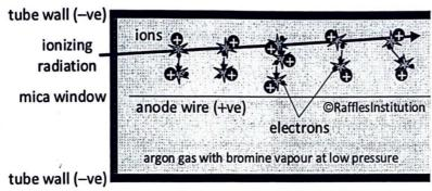
Fig. 20.23 A schematic diagram of a Geiger-Müller tube.
