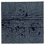
Tracks left by ionising particles in a cloud chamber.
