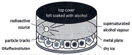
Fig. 20.22 A schematic diagram of a cloud chamber.
