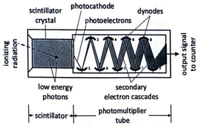
Fig. 20.24 A schematic diagram of a scintillation counter.
