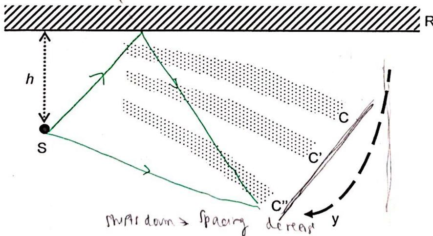
In the Appleton's experiment, S was a radio transmitter on the Earth's surface and R was the Heaviside layer – a reflecting layer in the atmosphere 80 km above the ground. When the transmitted wavelength is slowly changed from 200 m to 180 m, a receiver on the ground 120 km away from S observed fluctuations in the received signal strength. Calculate the number of signal maxima observed during this change of frequency.
