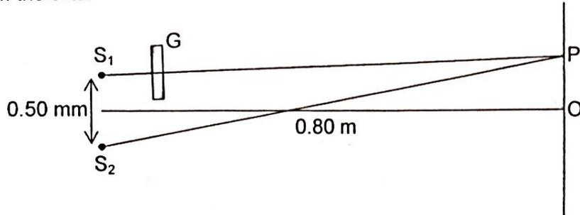
When a thin parallel-sided piece of glass G of thickness  $3.6 \times 10^{-6}$  m is placed in front of  $S_1$  as shown, the centre of the fringe system moves from O to a point P.
