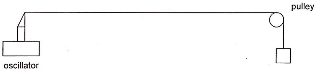
As the frequency of the oscillator is increased, stationary waves are produced on the string at certain frequencies.
