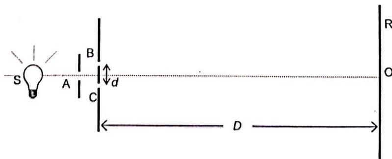
The figure above illustrates the Young's double-slit experiment. A source of light S illuminates a narrow slit A, which acts as a source for the narrow slits B and C, and produces fringes on the screen. With light of wavelength  $\lambda$ , bright fringes of separation  $s$  are formed on the screen. State the relation between  $\lambda$ ,  $s$ ,  $d$ , and  $D$ . Suggest suitable values for  $d$  and  $D$ .
