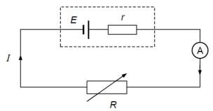
The resistance R is varied and the corresponding currents flowing through an ideal ammeter are recorded.
