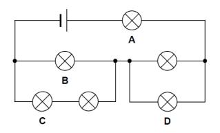
27 Five resistors of equal resistance are connected as shown.
