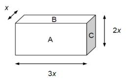
Electrical contact can be made to the opposite sides of the block. Between which two sides of the block should the electrical contact be made, so that the resistance of the block is a maximum?
