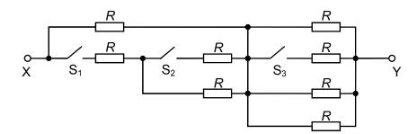
Which switch combination will give rise to the maximum total resistance between points X and Y?
