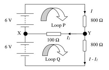
Using Kirchoff's Voltage Law, in loop P, we have  $6 = 800I + 100I_1 \dots (1)$ In Loop Q, we have  $6 = -100I_1 + 800(I - I_1) \dots (2)$ Solving equations (1) and (2), we have  $I_1 = 0$
