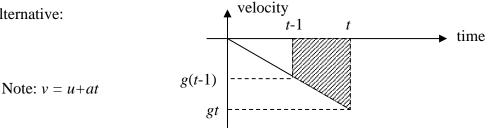
Let *s* be total distance covered and *t* the total time taken for the fall. Then the distance covered is the area under the velocity-time graph. We have  $s = \frac{1}{2}gt^2...(1)$
