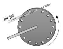
The time it takes for successive holes to move past the air jet is the period of the sound wave.
