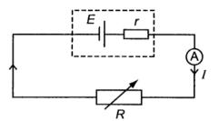
*R* is set at two different values and the corresponding currents *I* are measured using an ammeter of negligible resistance.
