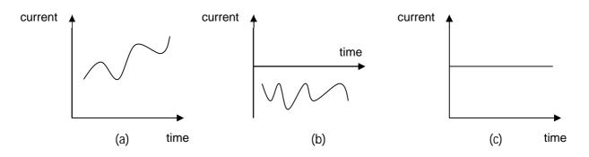
In (a) and (b), the magnitudes of the current change with time. The currents in (a) and (b) flow in the opposite direction. In (c), the current flows with constant magnitude. We say, the current is a steady D.C. This chapter focuses mainly on the type of current shown in (c) – steady D.C.
