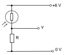
Determine the value R of a suitable resistor which can be placed in series with it so that the potential at Y changes from zero to 2 V when the LDR is illuminated. [Answer:  $600 \Omega$ ]
