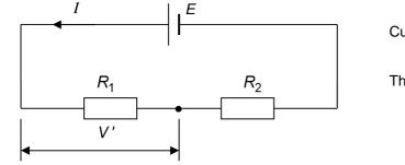
The potential difference V' is then connected to a load, such as a lamp.
