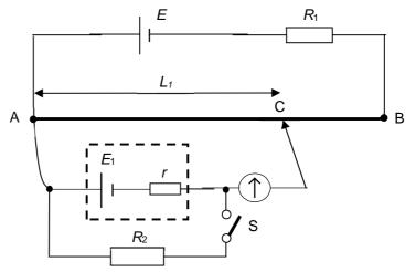
With switch S opened, no current passes through the loop containing the resistor of resistance  $R_2$ . The balance point is at point C and the balance length is  $L_1$ .
