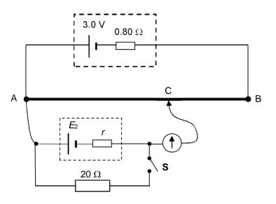
The movable contact C can be connected to any point along the wire AB. When switch S is opened, a balance length of 61.0 cm is obtained. When switch S is closed, a balance length of 49.5 cm is obtained. Find the internal resistance, *r*.
