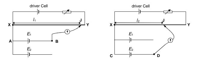
At the balance length (null deflection of galvanometer)
