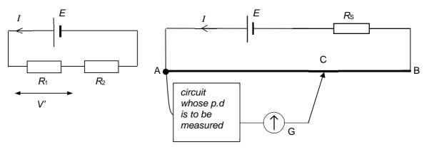
For a potentiometer found in our Physics laboratory, a length of resistance wire AB is used in place of the two resistors,  $R_1$  and  $R_2$ . An additional resistor  $R_s$  connected in series with the wire serves to limit the current that flows through the circuit. The resistance of  $R_s$  will affect the p.d across the resistance wire AB.
