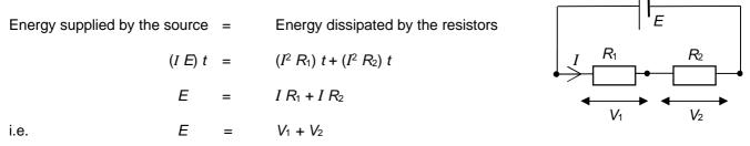
**Voltage Law**: In any closed loop in an electric circuit, the total e.m.f. *E* supplied equals to the total potential difference in that loop.
