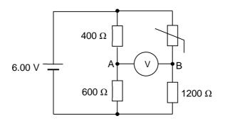
The voltmeter connected between A and B has infinite resistance. The battery has e.m.f. 6.00 V and negligible internal resistance.
