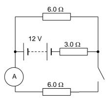
The switch is closed. [Answer: 1 A] Calculate the reading on the ammeter.
