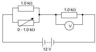
Calculate the maximum and minimum possible values of the voltmeter reading as the variable resistor is altered. [Answer: 12 V, 8 V] [N07/P1/29]
