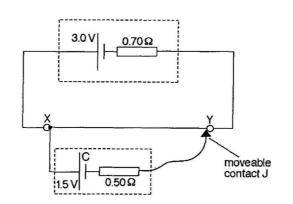
The moveable contact J can be connected to any point along the wire XY.
