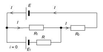
By changing the values of the resistors,  $R_1$  and  $R_2$ , we can change the p.d. across resistor  $R_1$ . When the p.d. across the resistor  $R_1$  is equal to  $E_1$ , no current will flow through  $E_1$ . We have now constructed a potentiometer, which is an arrangement which measures p.d. accurately.
