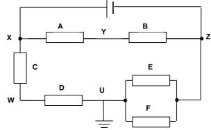
2. In the circuit, the battery has an e.m.f. of 12 V and an internal resistance of 3.0  $\Omega$ . The ammeter has negligible resistance.
