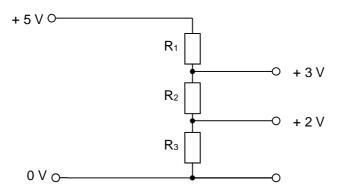
Which combination of resistances R<sub>1</sub>, R<sub>2</sub> and R<sub>3</sub> gives the correct voltages? [J96/P1/15]
