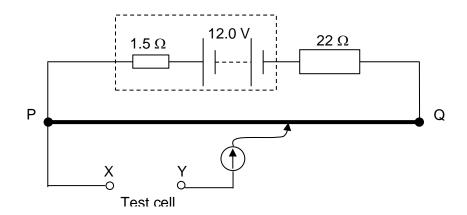
The wire PQ has a resistance of 3.0  $\Omega$  and the driver cell has an e.m.f. of 12.0 V. He was unable to obtain an observable balance length on PQ when he connected the circuit. The tutor he consulted told him that the test cell has an e.m.f. of a few millivolts. What could he do in order to obtain an observable balance length?
