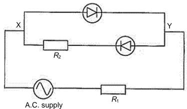
Which of the following graphs below represents the variation of current I with time t through  $R_1$  of the circuit in the diagram above?
