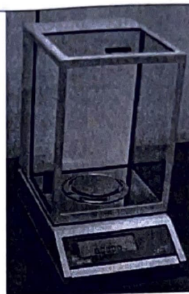
Figure 9b: Another type of analytical balance commonly used for weighing chemicals in the laboratory.
