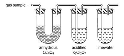
At the end of the experiment, it was found that the copper(II) sulfate was white, the acidified potassium dichromate(VI) was green and the limewater contained a white precipitate.
