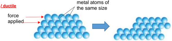
In an alloy, atoms are of <u>different</u> sizes, hence the regular arrangement of atoms is <u>disrupted</u>. Layers of atoms cannot <u>slide</u> easily over each other when a force is applied, and so an alloy is <u>harder</u> and stronger.
