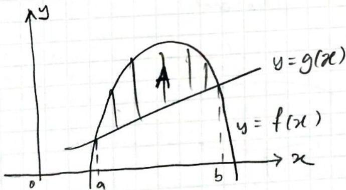
$$A = \int_a^b [f(x) - g(x)] dx \text{ if } f(x) \geq g(x)$$
