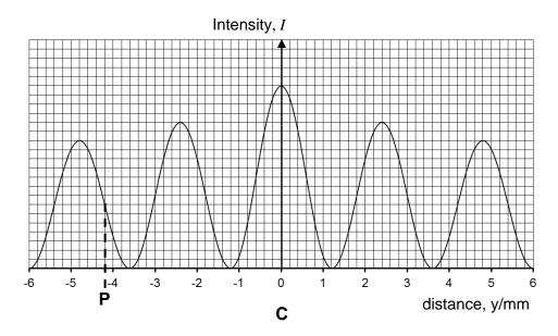
If **P** is a point on the screen and its position is indicated in the figure above, what is the phase angle between the waves from the double slit when the waves meet at **P**?
