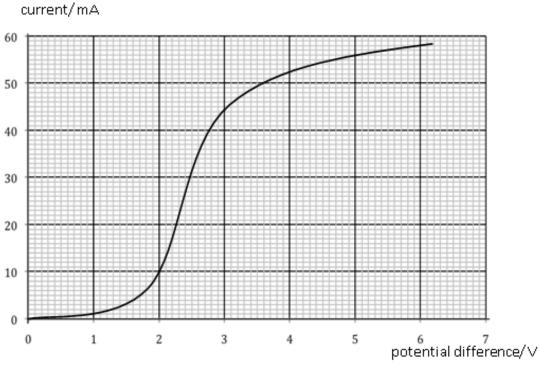
**23** A graph of current against potential difference for a component is given below.
