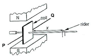
The coil is maintained in a vertical plane by moving a rider of mass M along a horizontal beam attached to the coil. When a current I flows through the coil, equilibrium is restored by placing the rider a distance x along the beam from the coil. What is the expression for B?
