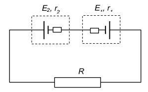
If the current flowing in the circuit is *I* and  $E_1 < E_2$ , what is the magnitude of the terminal p.d. across the cell  $E_1$ ?
