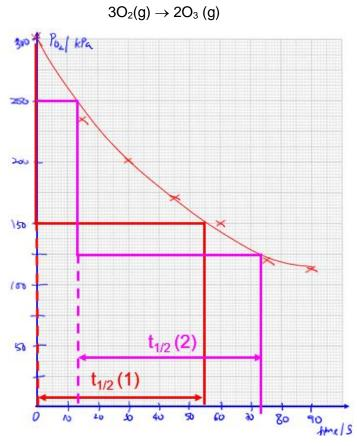
Determine the order of reaction with respect to oxygen
