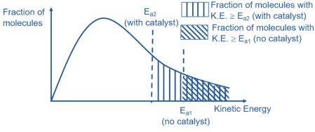
In the presence of catalyst, the reaction proceeds with an alternative reaction pathway of lower activation  $energy(E_a')$ .
