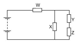
If the power dissipated by resistor Y is 3 W, what is the *total* power supplied by the battery?
